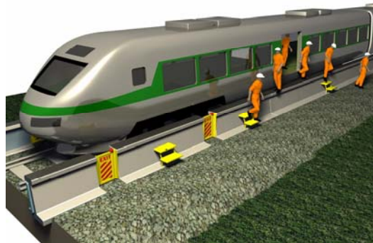
Figure 5. Low barriers to screen the noise produced at the wheel-rail contact point
