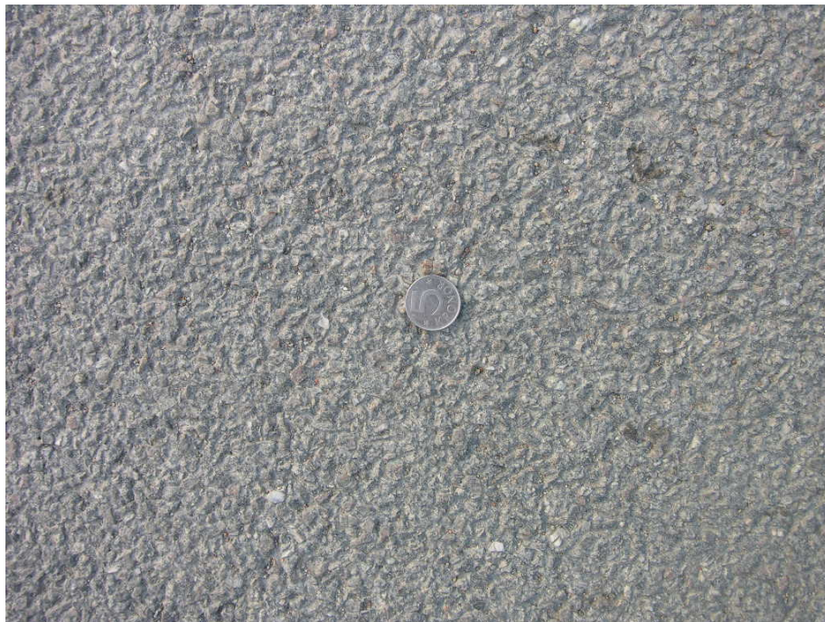
Figure 2. Close up photo (taken during the measurements) of the Thin Layer VIACOGRIP 8, with a Swedish 5 kronor coin as reference.
