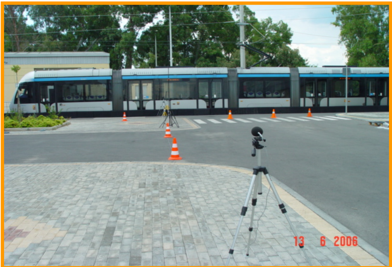
Fig. 5 Measurement's location setup for both "With" & "Without barrier" tests
