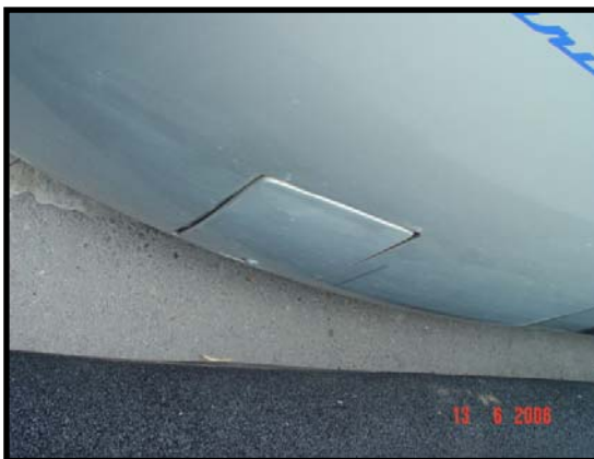
Fig. 4 Positioning of the CDM's barrier at Athens Tram Depot (at approx. 4-12cm from vehicle ext. gabarit)
