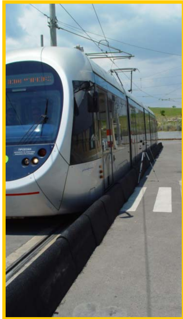
Fig. 4 Positioning of the CDM's barrier at Athens Tram Depot (at approx. 4-12cm from vehicle ext. gabarit)
