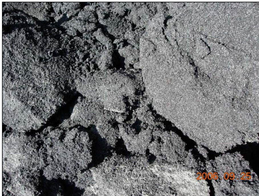
Figure 5. Rubber/bitumen mix in lumps before processing in ALLU (the biggest lump in picture is about 25 cm across).
